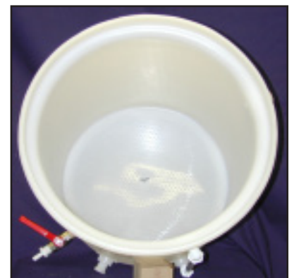
View of false bottom. Wing nut in center and support edge on perimeter
